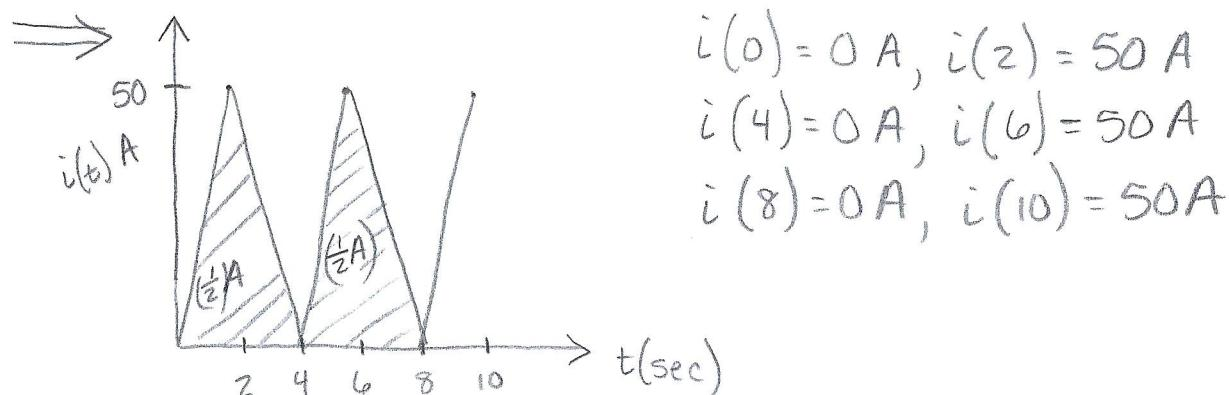
To find the total current through the circuit for  $0 \leq t(\text{sec}) \leq 8$  sec, determine area A for the interval  $0 \leq t \leq 8$
