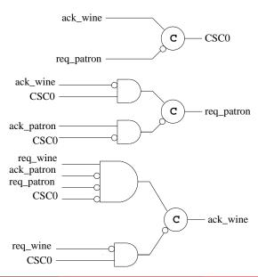
Note that req\_wine and ack\_patron are trigger signals for ack\_wine+.
